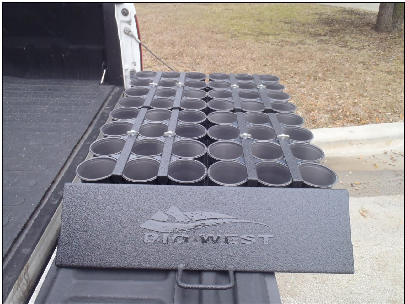
Figure 1. Mobile Underwater Plant Propagation Tray (MUPPT) prototype.
