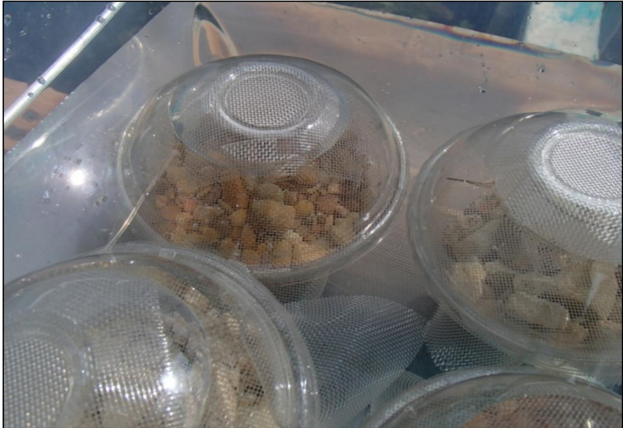
**Figure 46. Experimental enclosures for amphipod testing.**
