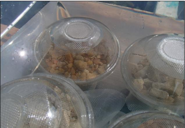
Figure 46. Experimental enclosures for amphipod testing.
