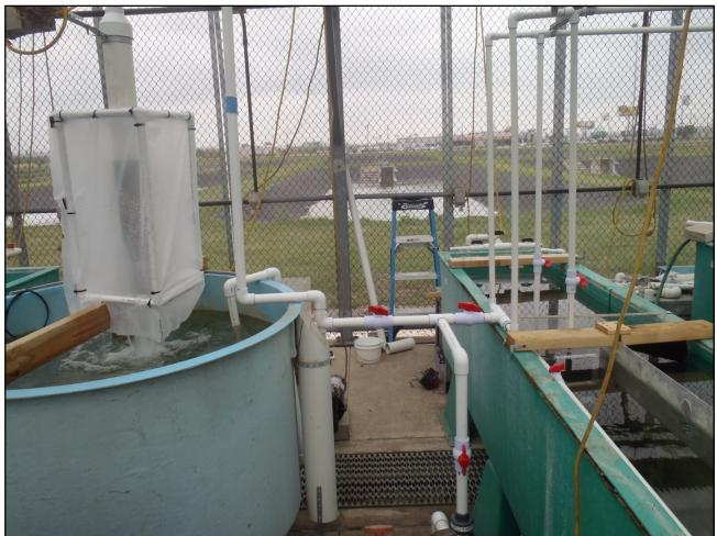
Figure 3. Reservoir Tank with CO2 degasser (left) and living stream divided in two right).
