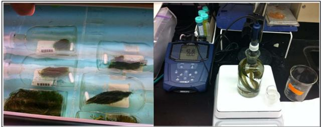
Figure 41. Subsamples of plant tissue were incubated in glass BOD bottles under lightsaturating conditions at controlled temperatures (left). Periodically, the bottles were removed and pH and dissolved oxygen (DO) levels measured (right).
