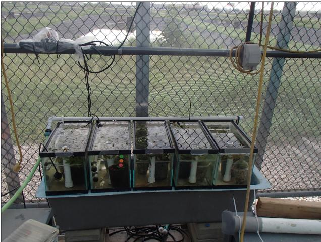
Figure 18. Pre-trial 1 equipment setup, including a five-tank array plumbed with various CO2 concentration and water temperature treatments.
