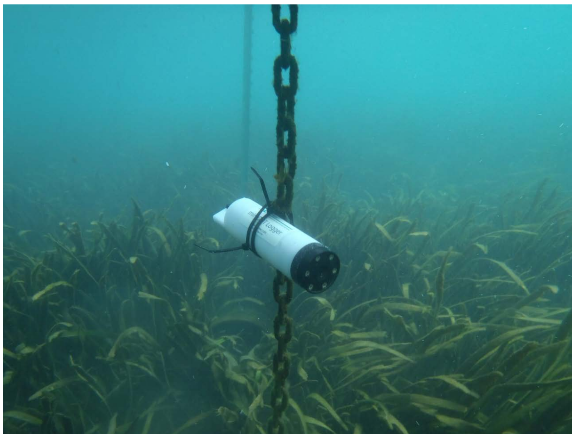
Figure 4.1 MiniDOT dissolved oxygen sensor deployed in Landa Lake during summer 2015.
