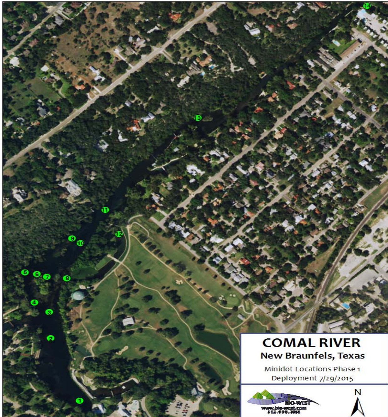
Figure 4.3 Location of 14 MiniDOT dissolved oxygen sensors during initial spatial evaluation study.
