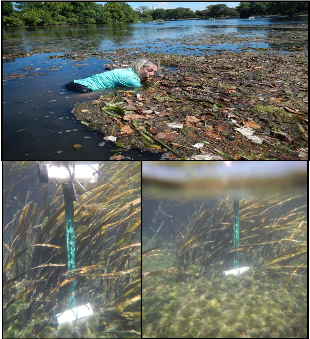
Figure 4.6 Top. Sarah Hester of Baylor University places MiniDOT sensors within the middle of floating vegetation mats. Mats are composed of a variety of aquatic and terrestrial debris. Bottom. Placement of MiniDOT sensors at the top and bottom of the water column. Note the dense bryophyte turf, composed of Riccia fluitans , located along the bottom.
