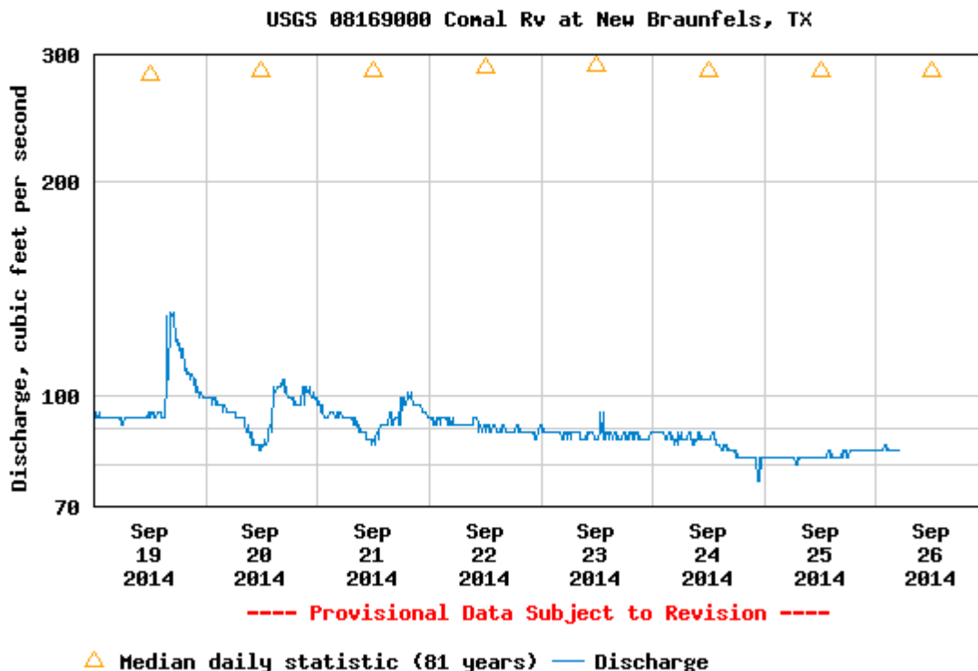
Figure 1: Screen shot of USGS webpage for the COMAL gage (08169000) showing total system discharge over the past week.
