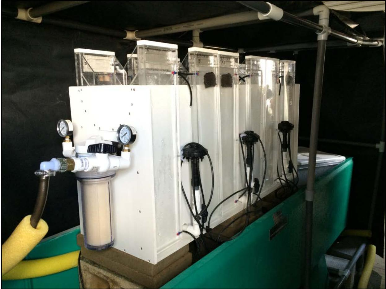
**Figure 3. Photograph of RBASS system setup at SMARC wet laboratory showing six RBASS environmental flow chambers, upwelling flow spigots, black nylon cover, and inlet water line. The refugia tank can be seen at the far end of the green fiberglass living stream.**
