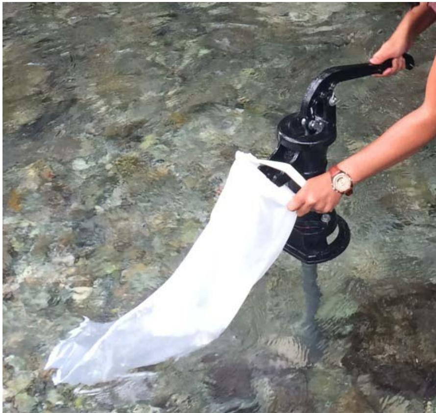
**Figure 9.** Picture of a Bou-Rouch pump used for collections along Comal SR3.
