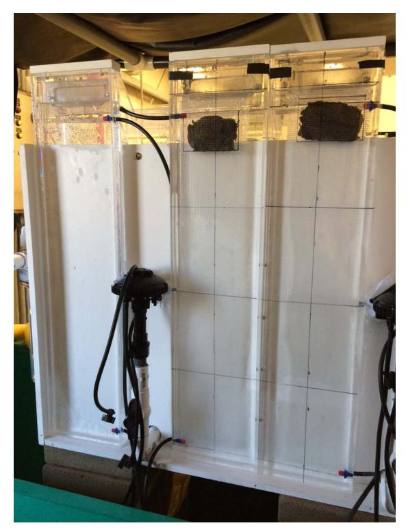
Figure 6. Photograph of EFC with surface organic layer (SOL), EFC inlet (bottom diffuser cap), EFC outlet (middle diffuser cap), and grid overlay.
