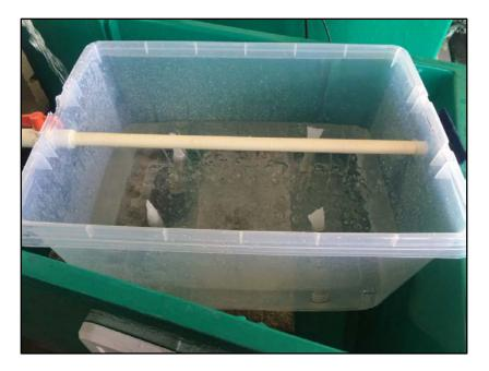
Figure 2. Refugium tank, showing water flowing in through the top and draining out through the bottom, with rock and leaf substrates.
