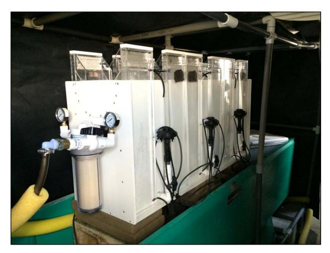
Figure 3. Photograph of RBASS system setup at SMARC wet laboratory showing six RBASS environmental flow chambers, upwelling flow spigots, black nylon cover, and inlet water line. The refugia tank can be seen at the far end of the green fiberglass living stream.
