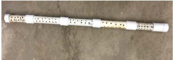
Figure 7. Picture of the passive sampling pits utilized to examine the vertical and lateral distribution of riffle beetles in Comal SR3.
