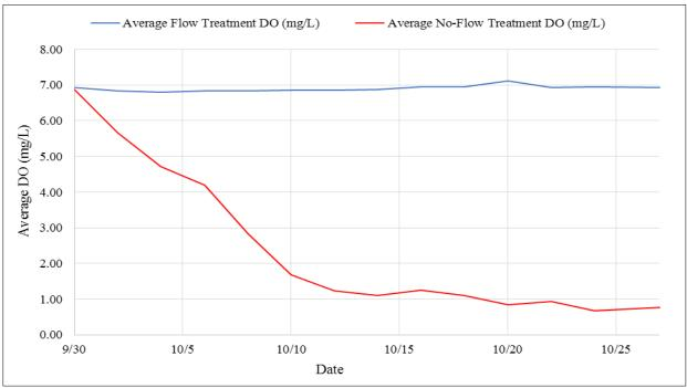
Figure 9. Time series plot of environmental flow chamber DO (mg/L) over course of experiment.
