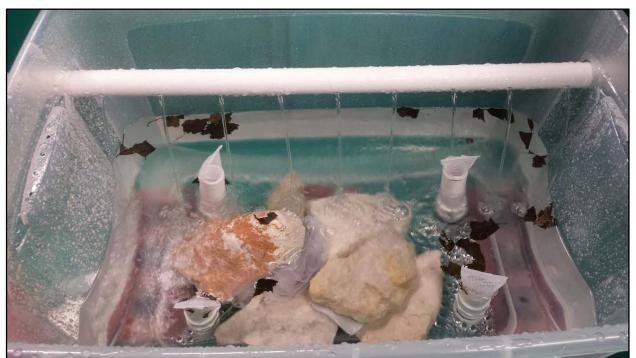
Figure 1. Refugium tank, showing water flowing in through the top and draining out through the bottom, with rocks, mesh and leaf substrate.
