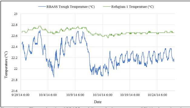
Figure 11. Time series plot of RBASS outfall vs. refugia temperature (°C) 10-minute thermistor data over course of experiment.
