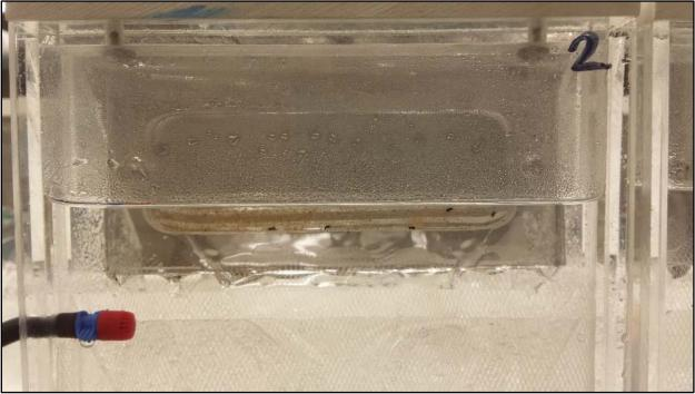
Figure 13. Photograph of beetles (dark dots) and waterline on fine mesh spillover screen at top RBASS environmental flow chamber. Beetles in this image are situated below the waterline.
