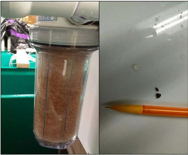
Figure 7. Photographs showing large and small iron oxide particulates found in RBASS unit water system.
