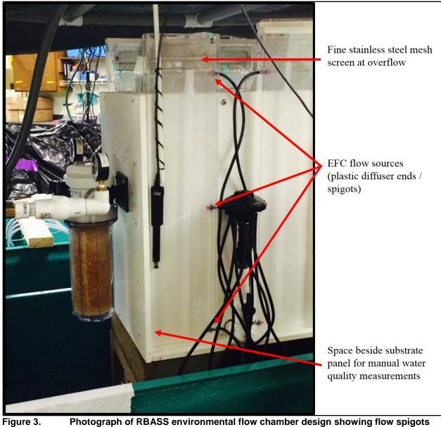
Photograph of RBASS environmental flow chamber design showing flow spigots and mesh screen at chamber overflow point.
