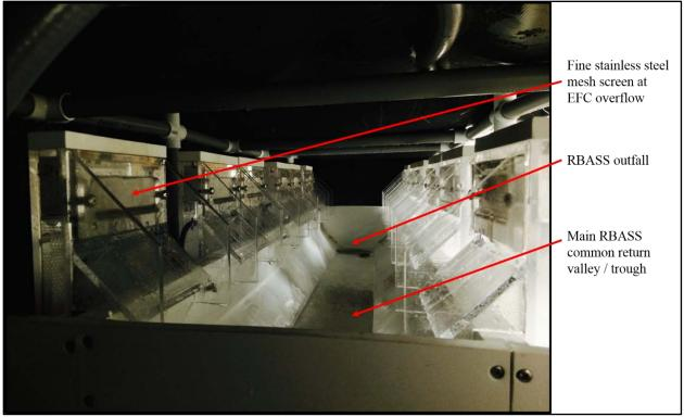
Figure 4. Photograph of RBASS trough/valley design showing interior sides of mesh screen at chamber overflow point.
