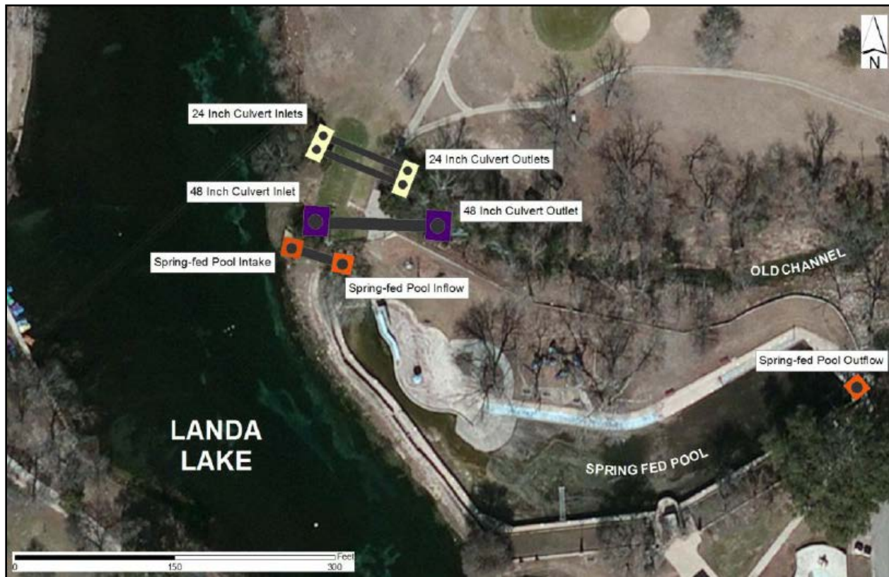
Figure 3-3. Locations of culverts for flow-split management (HDR 2013).
