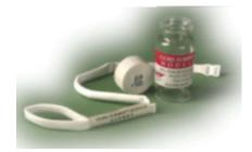
Figure 5. Universal Passive Sampler and Its Glass Vial (ITRC, 2005)
