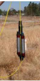
Figure 4. Rigid Porous Polyethylene Samplers (ITRC, 2005)
