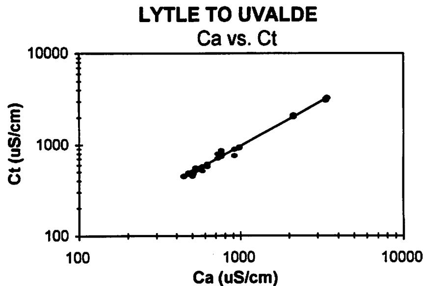
**Figure 5.** Correlation between measured specific conductance ( $C_t$ ) and geophysical log-derived specific conductance ( $C_a$ ) for control wells (Table 3). Specific conductance in microsiemens/cm.
