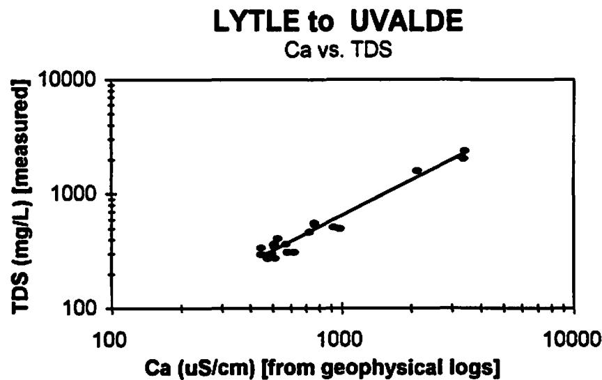
**Figure 6.** Correlation between measured total dissolved solids (TDS) and specific conductance (Ca) calculated from geophysical logs of control wells (Table 3). Crossplot reveals a well defined trend and a high correlation coefficient squared ( $r^2$ ) = .979. Total dissolved solids in mg/L. Specific conductance in microsiemens /cm. Relationship is: TDS estimated (TDSest.) = .67Ca - 12.
