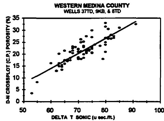
**Figure 3.** Plot of density-neutron log-derived porosity versus interval transit time, used to derive empirical relationship for determining porosity from 3 sonic logs in western Medina County. Relationship is:
