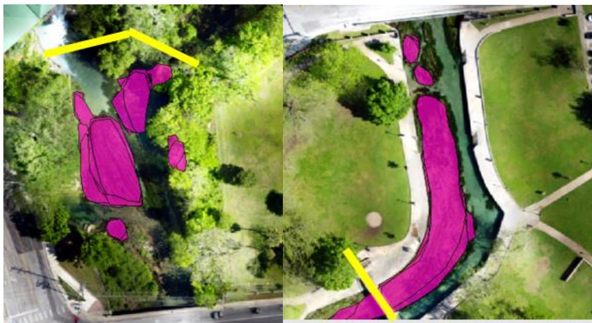
Figure 4. Areas in pink show the normal location for vegetation mat accumulation that were removed to quantify buildup on a weekly basis. Yellow lines mark the boundaries of the collection area. Spring Lake Dam Reach on left. Sewell Park Reach on the right.
