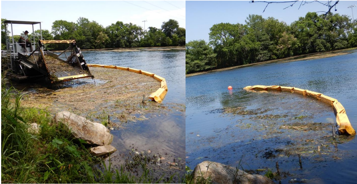
Appendix A1. The harvester emptying out temporary boom 3 after additional anchor weights were installed and subsequent leftover vegetation due to shallow water inhibiting the harvester's access.
