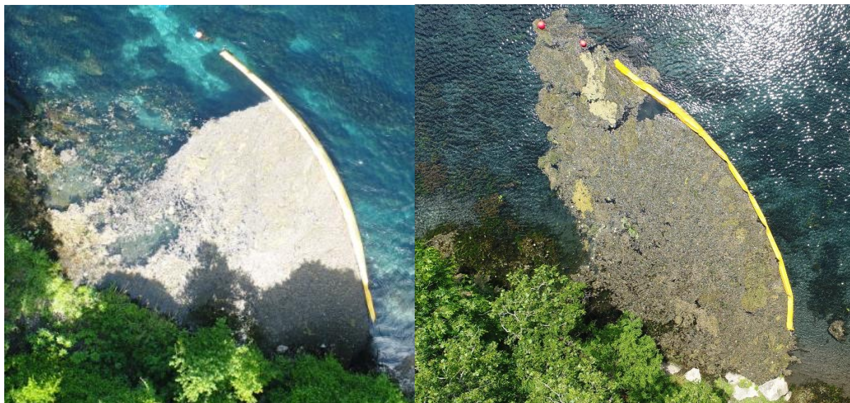
Figure 5. Aerial imagery shows boom 2 at full capacity before vegetation started to flow underneath the skirt (Left). Imagery of boom 3 shows that it was able to hold more at full capacity, with vegetation extending out past the opening (Right).
