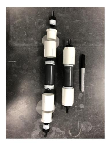
**Figure 1**. Structure and size of an upwelling flow-through chamber used in the air space access experiments. Note the pieces of 100 mm Nitex mesh used at the ends to prevent escape or loss of CSRBs.
