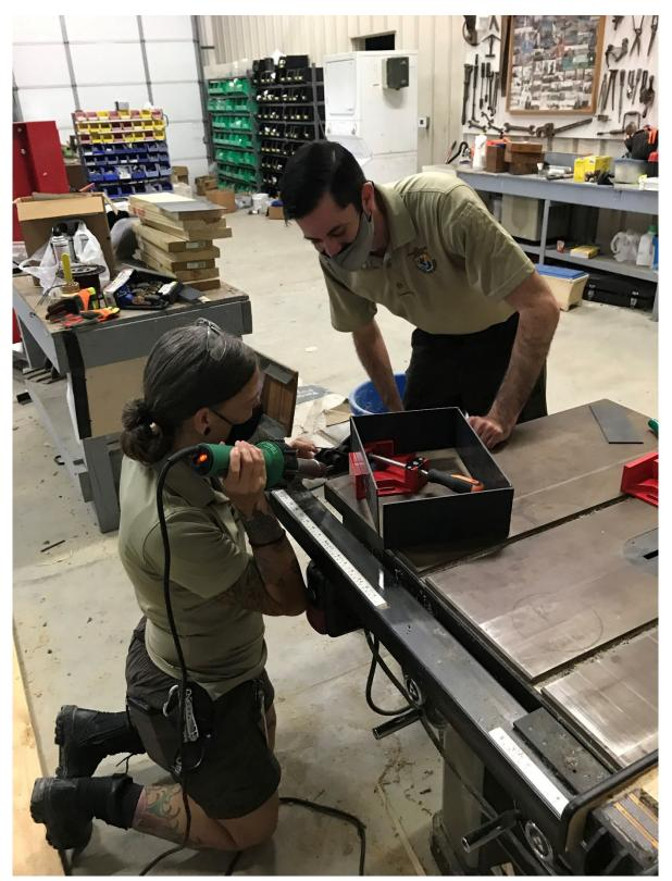
Figure 3. Jennifer Whitt heat welding the corner seams on the filter box that was added to the redesigned invertebrate rack with Adam Daw's supervision.
