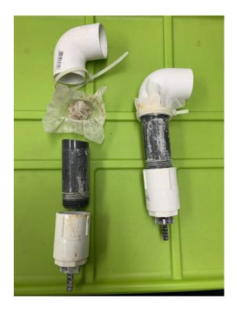
**Figure 2**. Structure and size of an upwelling flow-through chamber that maintained an air-water interface used in the air space access experiments. Note the pieces of 100 mm Nitex mesh used at the ends to prevent escape or loss of CSRBs and to create an air-water interface.
