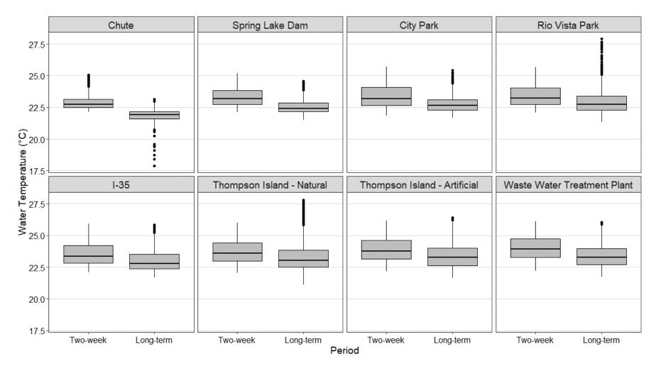
Boxplots comparing recent two-week and long-term water temperature trends at eight monitoring stations from Chute to Waste Water Treatment Plant for the month of June 2023. The thick horizontal line in each box is the median and the upper/lower bounds of each box represents the interquartile range. Whiskers represent minimum/maximum values up to 1.5 times the interquartile range, and outliers beyond this are designated with solid black circles.
