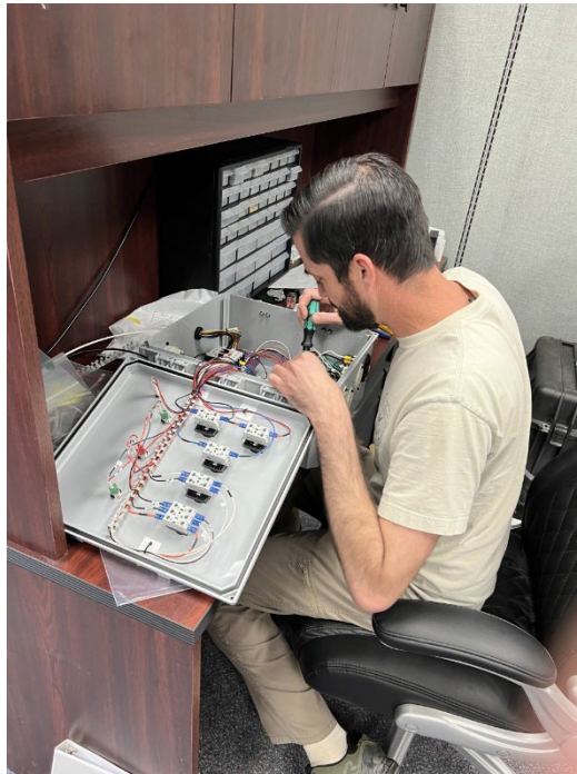
Figure 2. Adam Daw wiring the electrical panel for the new control/monitoring system.
