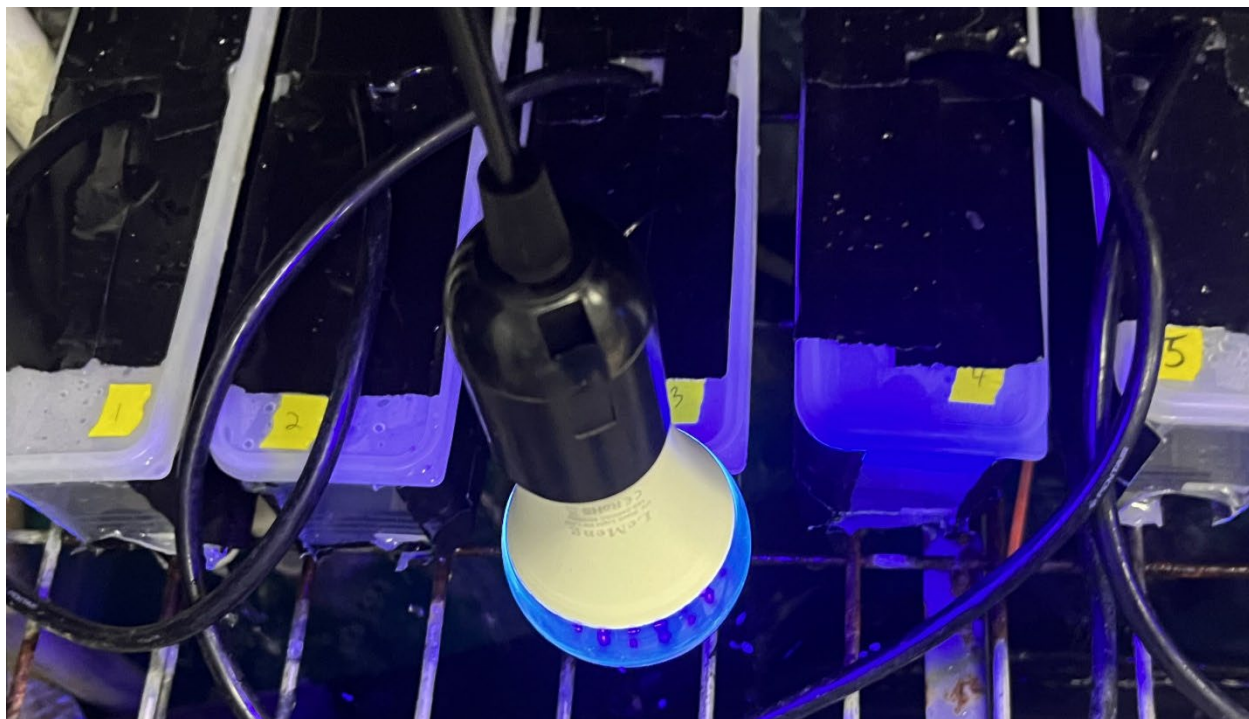
Figure 4. Photo showing experimental setup using chambers illustrated in Fig. 1 during an experiment testing beetle responses to ultraviolet (UV) light. In this experiment, the chamber was blacked out to prevent light from entering from all sides except the end with the lights above, while the entire setup was covered in black plastic to prevent other light sources in the room from influencing activity in the chambers.
