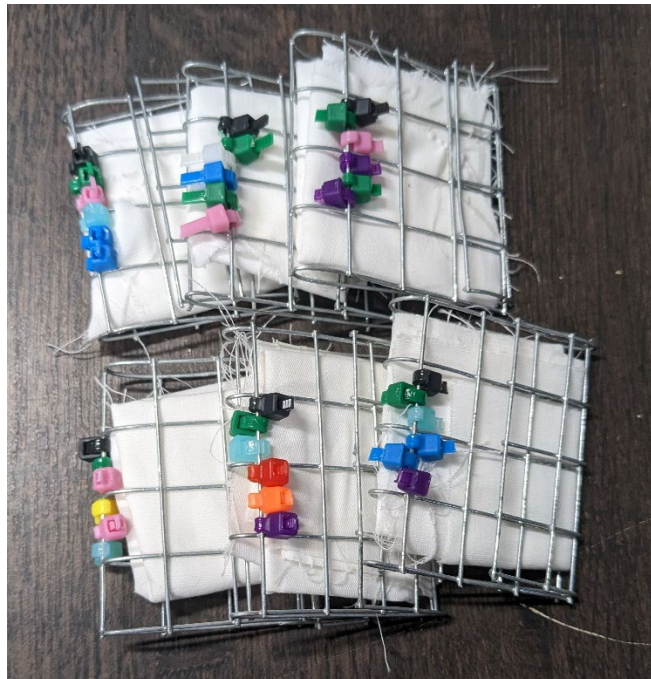
Figure 4. Poly-Cotton lures with color coded barcodes for unique identification in the field. Barcode starting position is designated by the black zip-tie.
