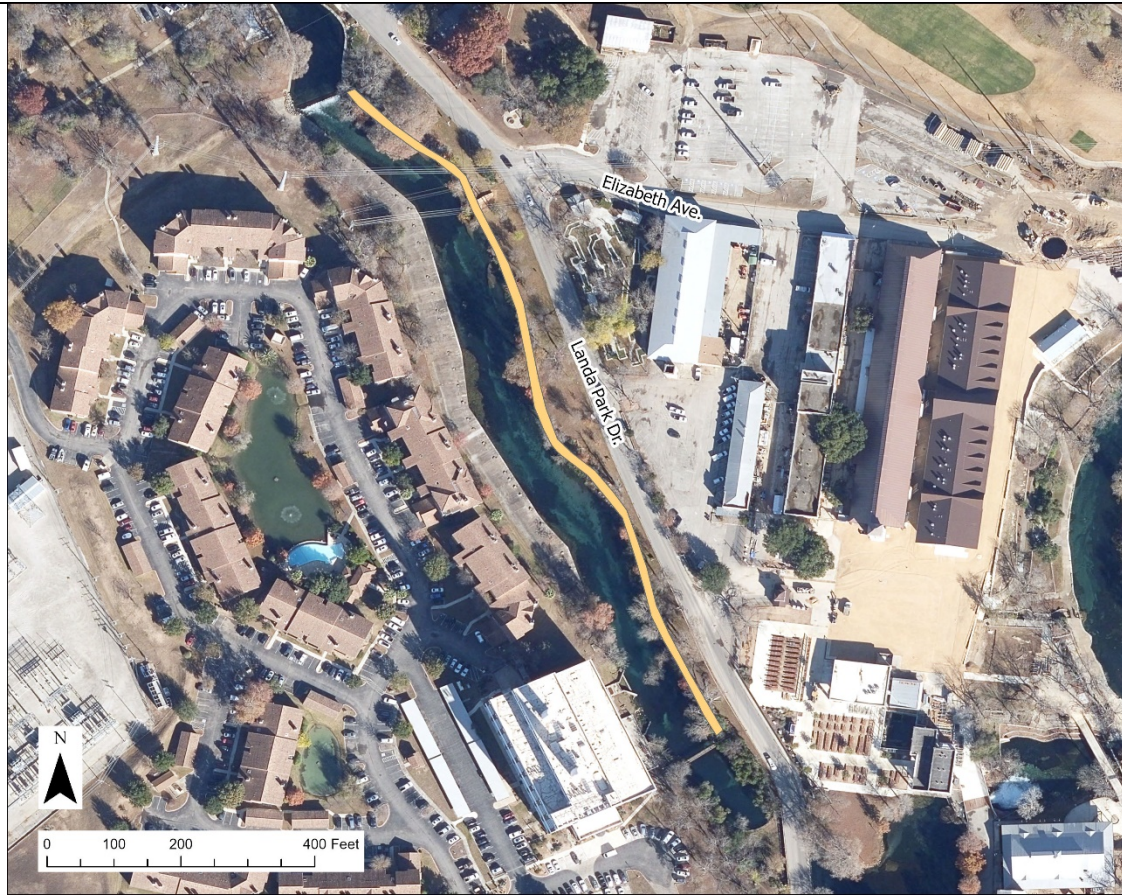
Figure 2. Location of 2023 riparian restoration along New Channel/ Mill Race of the Comal River. Restoration in this area to include removal of non-native vegetation, installation of erosion/ sediment control berms, and planting of native plants.
