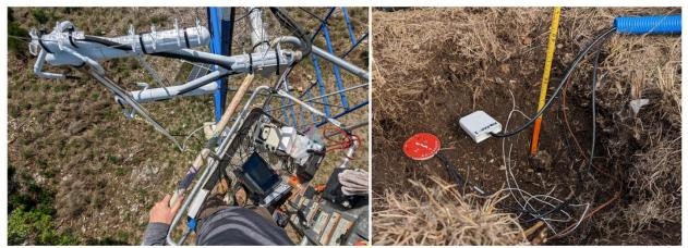
**Figure 2.3 Field Photographs of Cibolo (US-EA4) Station Maintenance.** (left) UT-BEG personnel performing a zero-span on the Cibolo station IRGASON from a lift; (right) installation of ground-based sensors in soil pit #2 at the Cibolo site during the site upgrade in January 2023.
