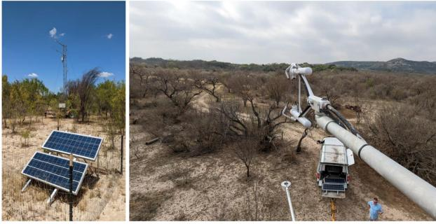
**Figure 2.4. Field Photographs of Uvalde (US-EA5) Station.** (left) Eddy covariance station at the Uvalde site; (right) photograph of the Uvalde site looking approximately into the direction of the sonic azimuth showing general characteristics of mesquite woody savanna ecosystem within measurement footprint (photograph taken in February 2023 during leaf-off conditions).
