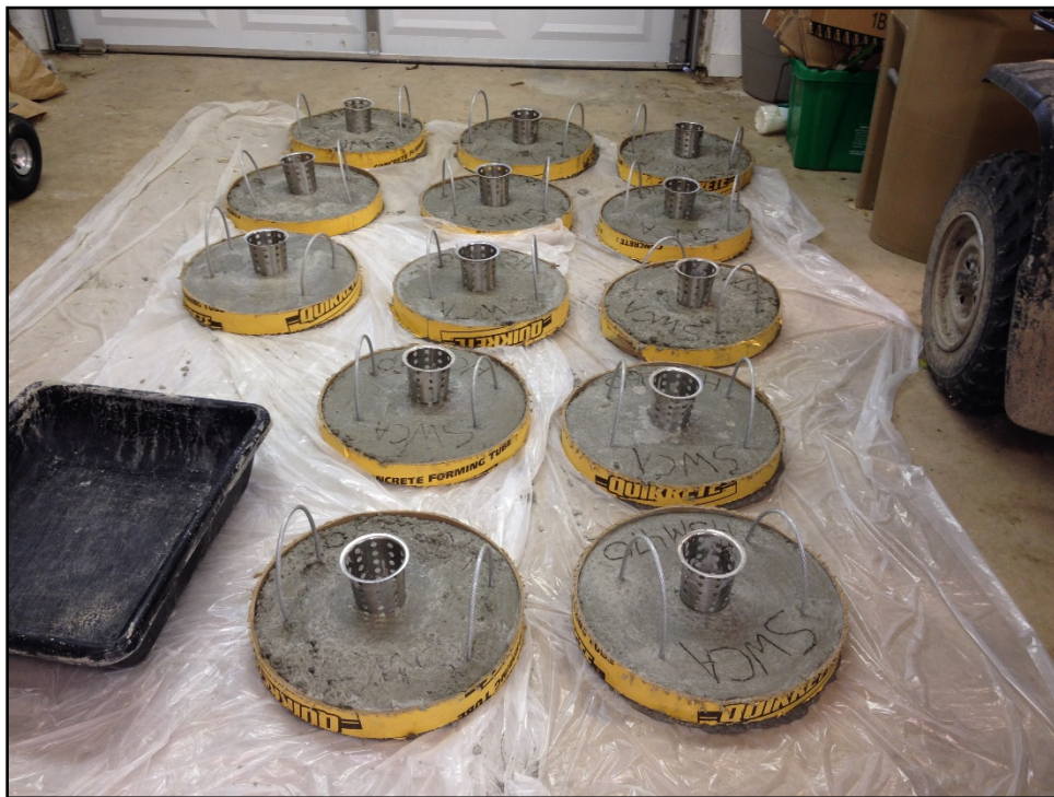
PHOTOGRAPH 16. Construction of PDS deployment devices.
