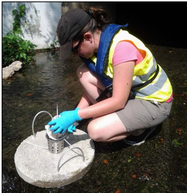
Figure 11. PDS deployment device prior to installation at site HSM440.
