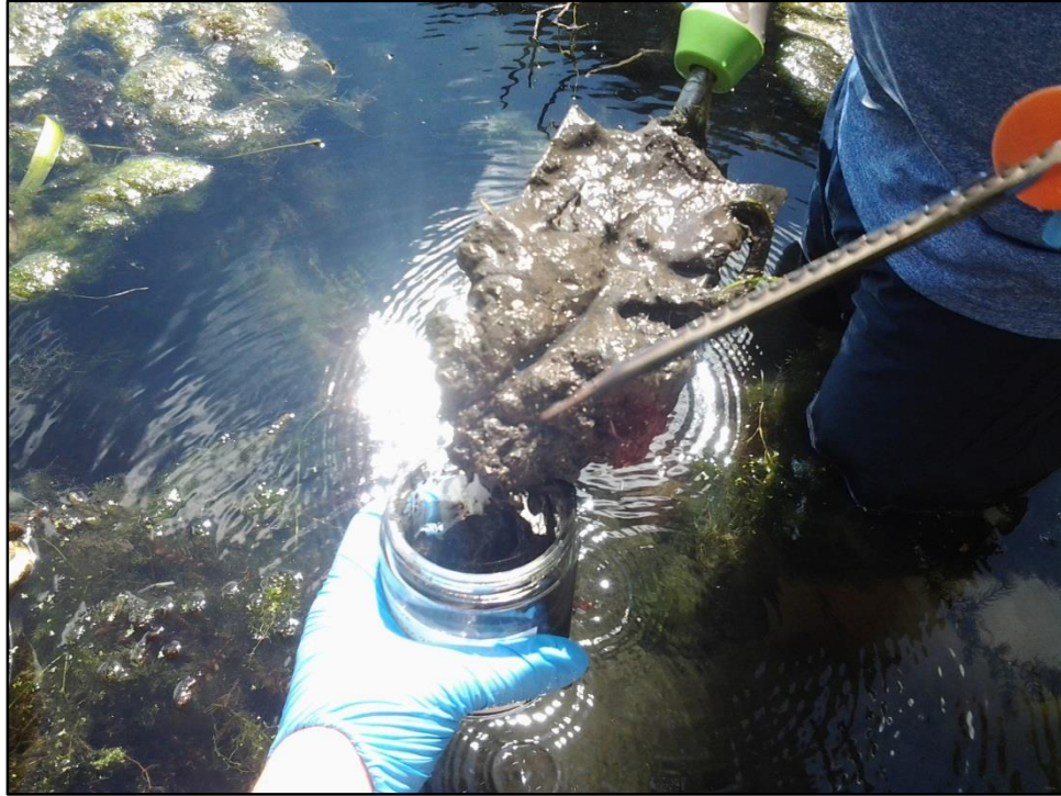
PHOTOGRAPH 7. Sediment sample collected with trowel, June 5, 2015; sample location HSM320.
