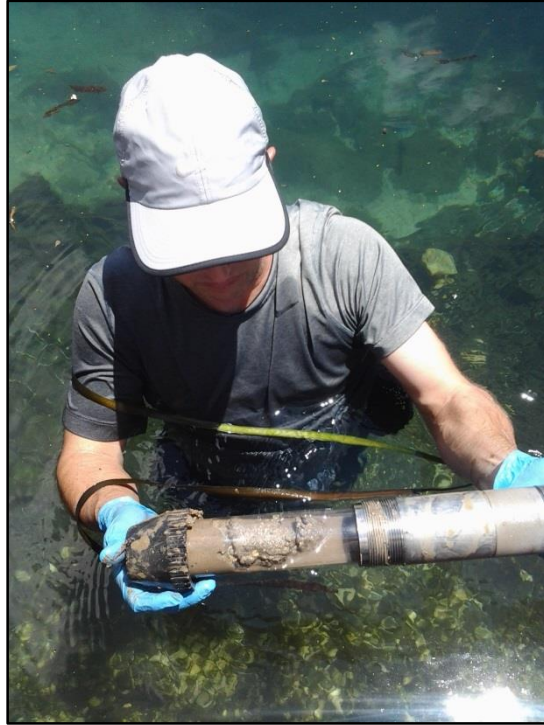
PHOTOGRAPH 5. Sediment sample collected with core sampler, June 4, 2015; sample location HCS330.
