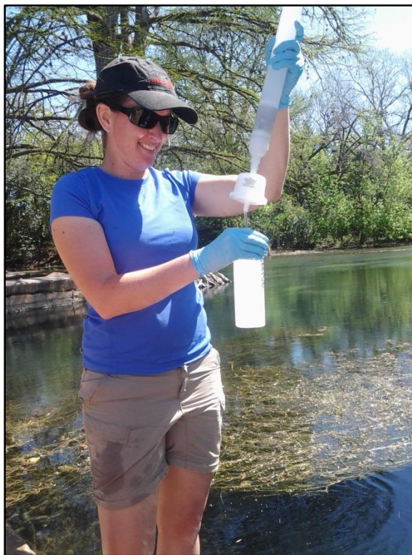
PHOTOGRAPH 2. Field filtering surface water grab samples, March 24, 2015; sample location HSM150.
