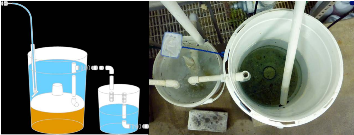
Figure 5 Picture of a amphipod separation system. Muck from the bottom of a pond is placed into a bucket fitted with a drain pipe mounted on the side. A cover made from the top of a 19l water jug is placed over the muck. Fresh water is pumped into the bucket over the cover. Amphipods and other organisms fleeing anoxic conditions under the cover swim up and are flushed out the drain pipe into the second bucket where they can be collected.
