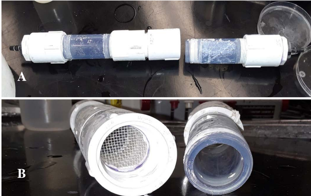
Figure 7 (A) Flow-through separation chambers with clear threaded PVC and (B) mesh screen for the separation of the young. Picture courtesy of Bio-West.
