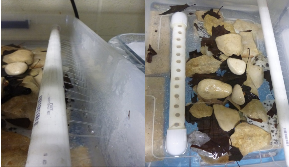
Figure 3. Inner construction and design of an easy spring container. (Left) Spray bar extends to the container wall before trickling to the water line. (Right) Rocks are spaced far enough to allow water to flow between the stacks to prevent anoxia.
