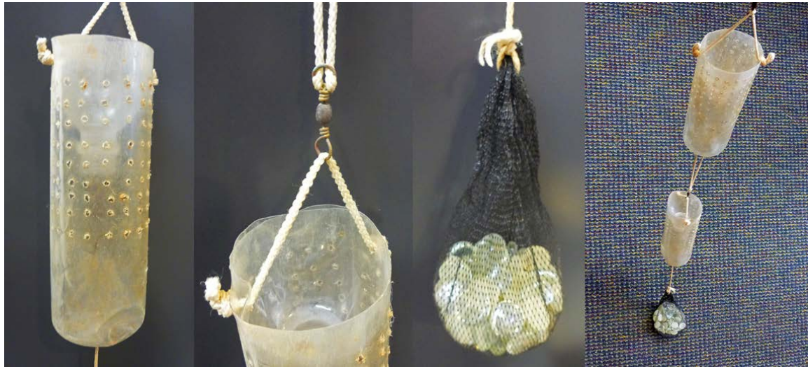
Figure 3 Bottle trap design for collecting salamanders.
