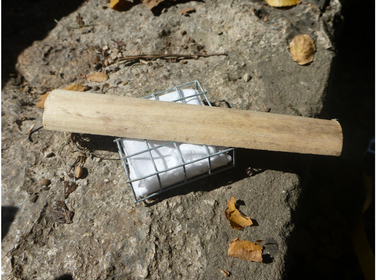
Figure 3 Cloth lure and wooden dowel before biofilm has developed.
