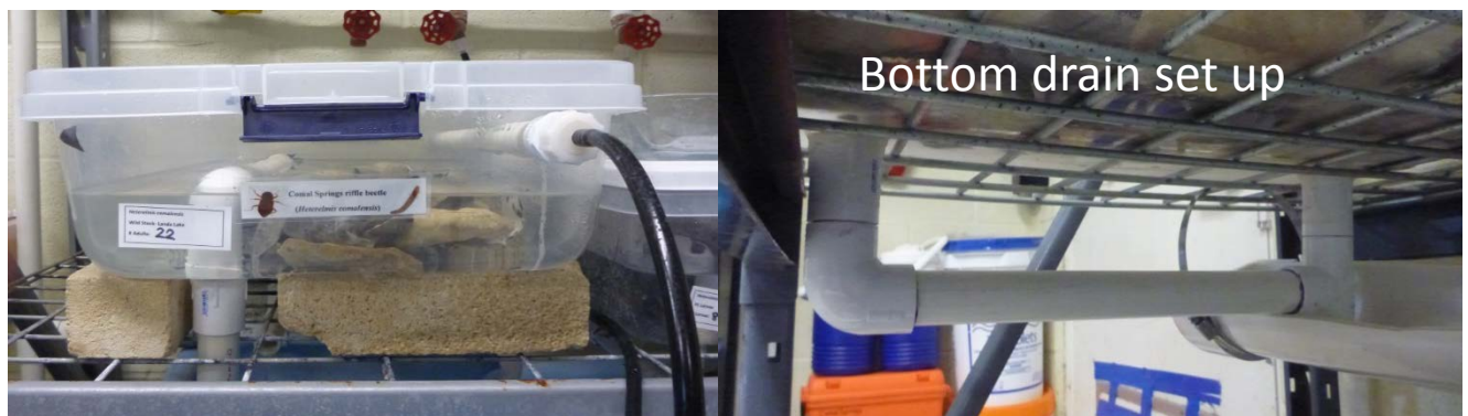
Figure 2 Outer construction and design of an easy spring container. Outflow design is one of many options and can be changed to fit your refugia preferences
