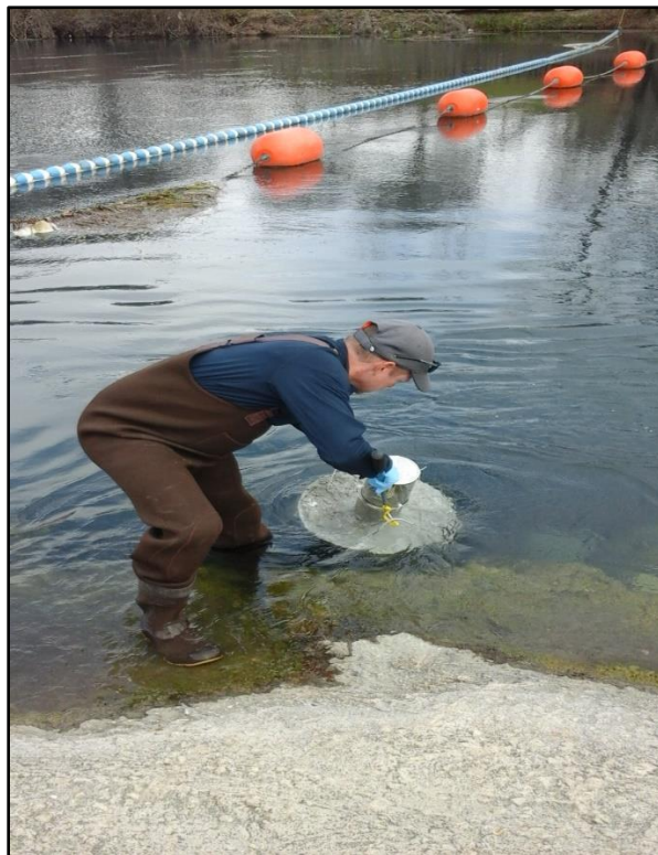
Photo 6. Installing POCIS on February 1, 2017; Sample location HCS460
