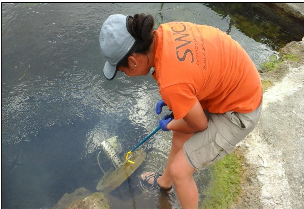
Photo 3. Placing PDS Deployment device using hook; August 1, 2017; Sample location HCS460
