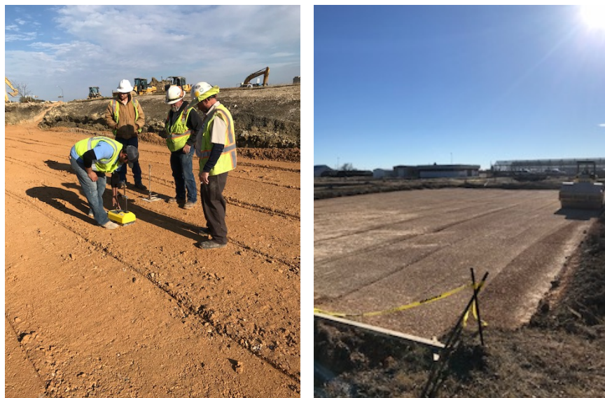
Figure 2. (Left) testing lab personnel using a nuclear densitometer to measure density and moisture content of testing area. (Right) Finished product
