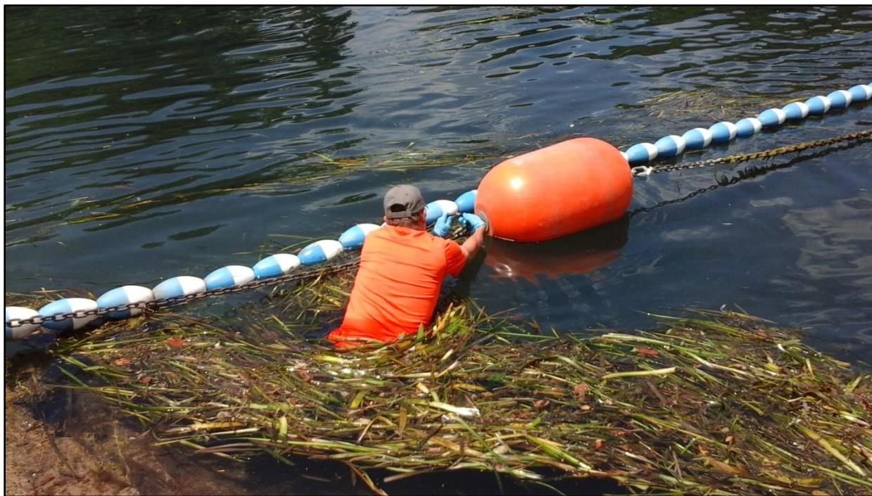
Photo 3. Locking the POCIS stainless-steel encasement sampler onto the chain with buoys that spans the Comal River at HCS460.
