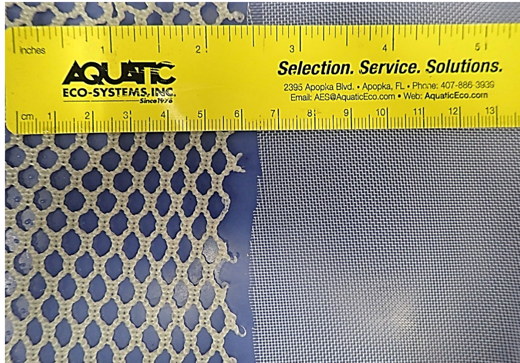
Soft netting for transport (cushioning, grips for babies) versus stiff mesh (750 micron)
