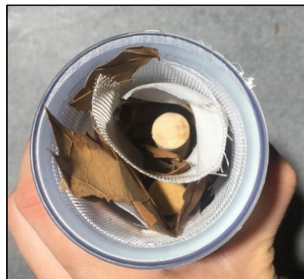
Figure 2 Flow-through tube design with cloth and leaves. The poplar wood dowels seen in this picture will be replaced with either balsa wood or roots. Pictured here is from a prototype in 2017. Current mesh is much larger in size and reinforced on the edges to reduce fraying.
