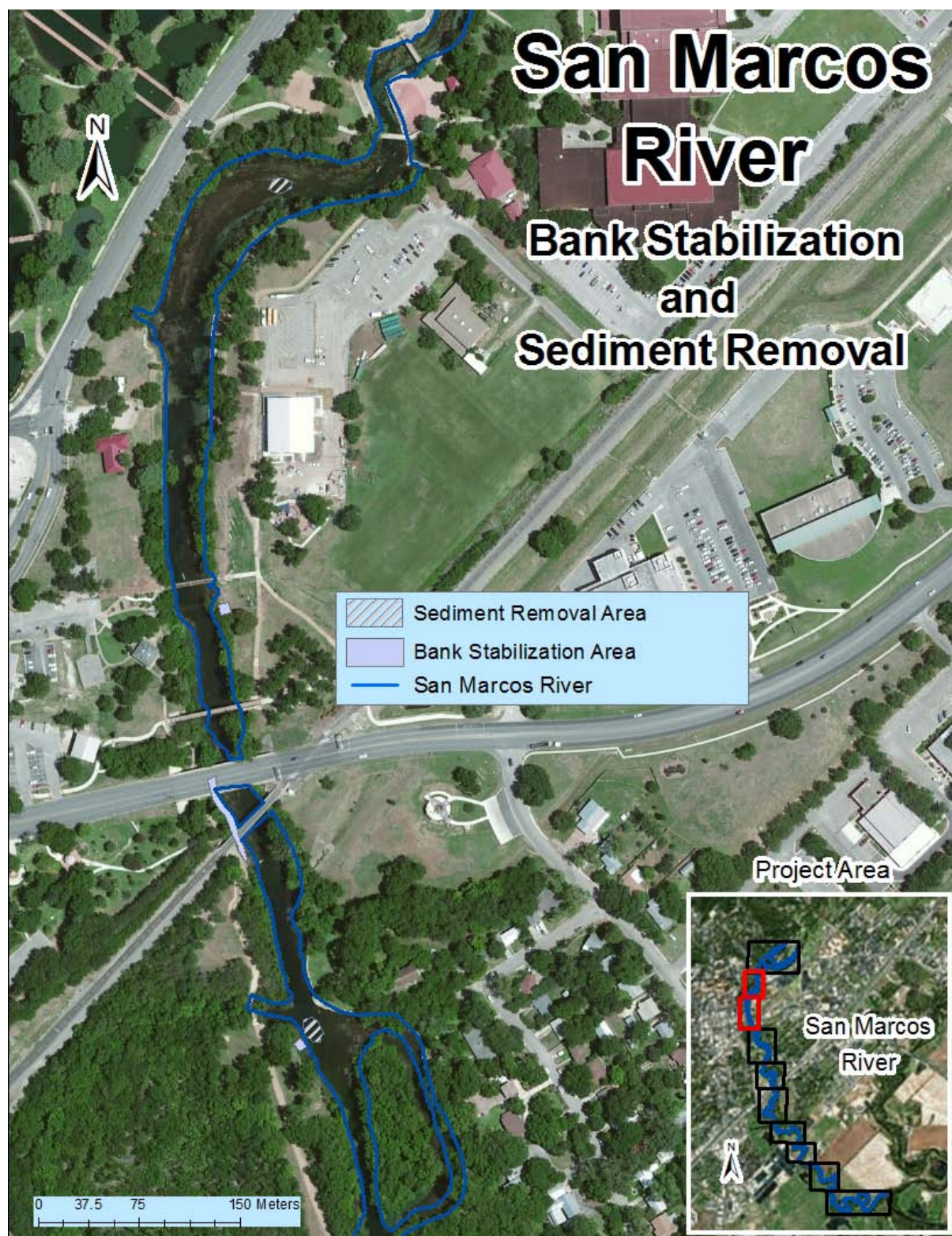
Figure 18: 2014 Sediment Removal and Bank Stabilization areas – San Marcos River.
