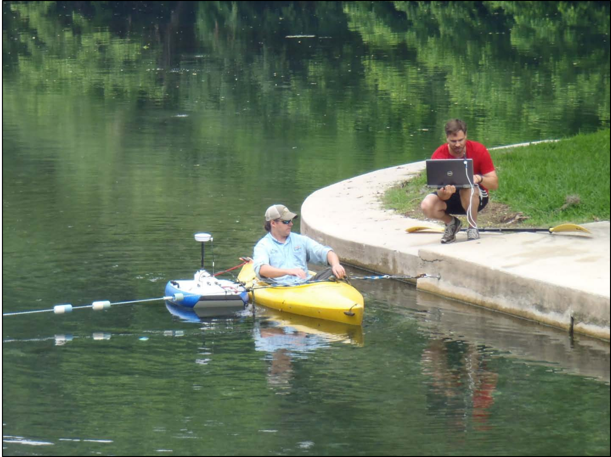
BIO-WEST biologists using a SonTek® RiverSurveyor M9 Acoustic Doppler Current Profiler to collect flow measurements near Spring Island in April 2015.
