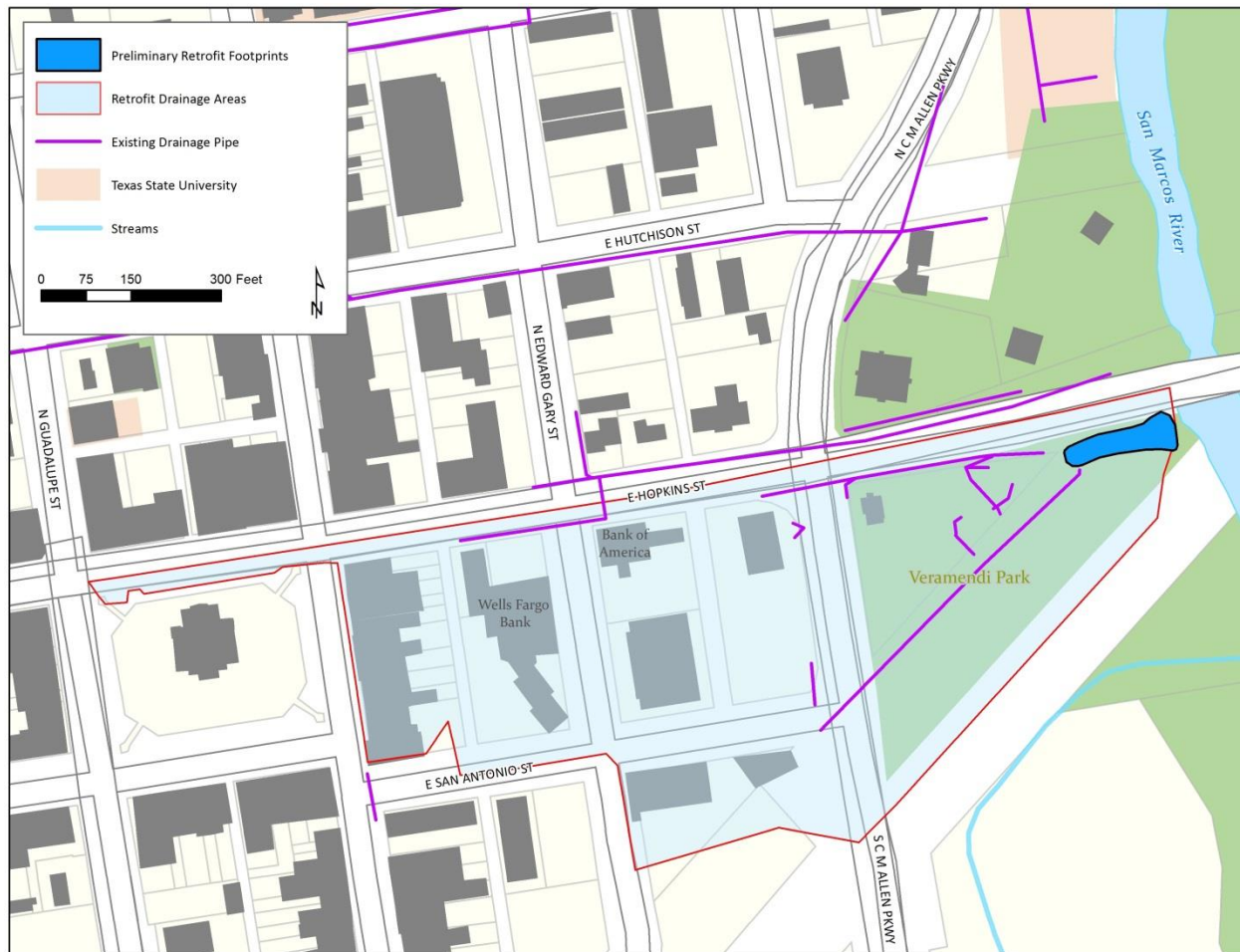
Figure 8-27 Hopkins Drainage Channel Pond 2 Retrofit: Concept Plan
