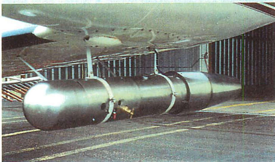
Figure 4: An acetone generator on a Cessna 340 aircraft.
