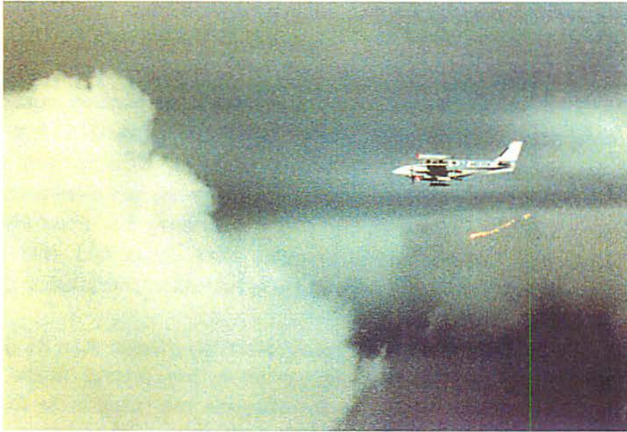
Figure 3: A cloud seeding aircraft dropping ejectable flares at cloud top (photo courtesy John Ulan).
