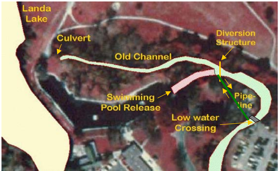
Figure C-14. Overview of recommended refugia in upper section of Old Channel Reach. A pipeline would recapture a portion of in-stream water from below the low-water crossing (path to golf course) and bring it back upstream to the diversion structure during low flow to increase water quantity in about 100 meters of high quality fountain darter habitat. The diversion structure and pipeline would also allow water to be routed around the area during high-flows for experimentation. The approximately 100-meter long habitat could also benefit from restoration activities designed to remove lower quality vegetation and increase vegetation that provides high quality fountain darter habitat. Comal Springs riffle beetle habitat could also potentially be created in this area.
