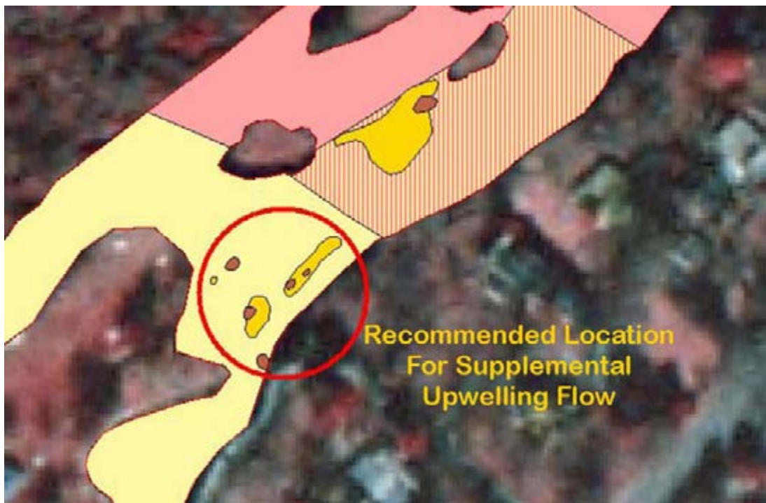
Figure C-9. Close-up of Comal Springs riffle beetle habitat upstream of Spring Island. These habitats are formed by upwelling springflow, which supplemental water should attempt to simulate. If introduced as surface flow, the supplemental water would not be as beneficial in this area. Areas within the red circle should receive highest priority for water supplementation.
