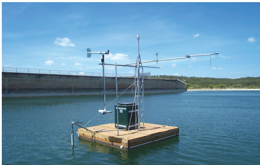
Figure 4. Weather station on Medina Lake, Texas, March 2001.
