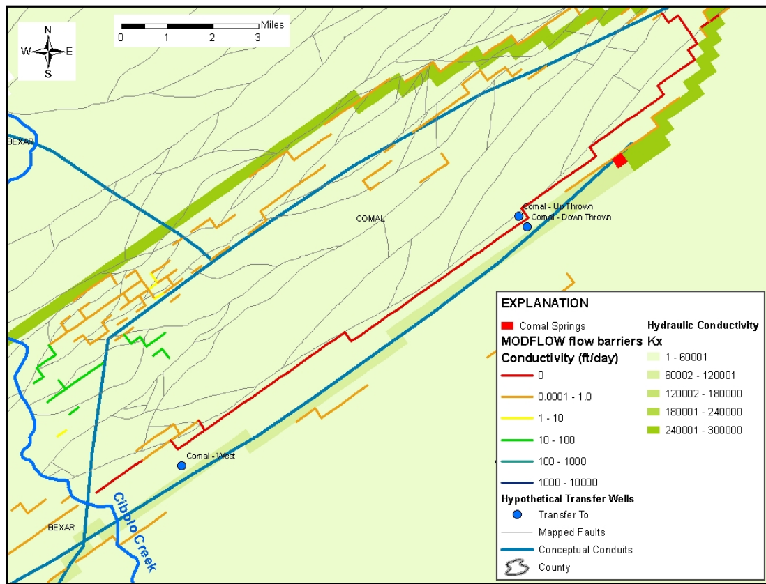
Figure 3.1 Location of Actual and Simulated Faults near Comal Springs
