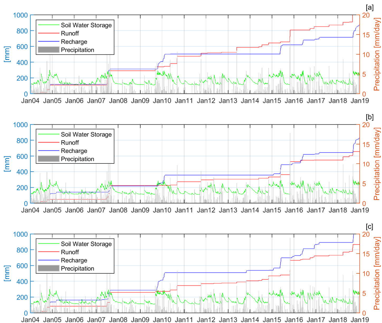
Figure 3-18: HYDRUS simulations of cumulative fluxes of runoff and diffuse recharge (Recharge), and precipitation rate and soil water storage at the [a] Woodland, [b] Savanna, and [c] Grassland eddy covariance sites.
