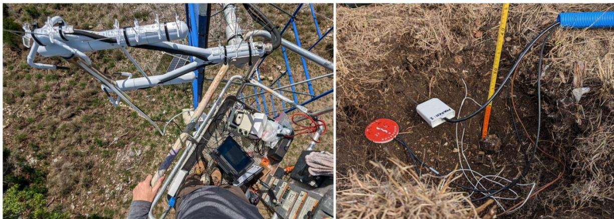
**Figure 2.3 Field Photographs of Cibolo (US-EA4) Station Maintenance.** (left) UT-BEG personnel performing a zero-span on the Cibolo station IRGASON from a lift; (right) installation of ground-based sensors in soil pit #2 at the Cibolo site during the site upgrade in January 2023.
