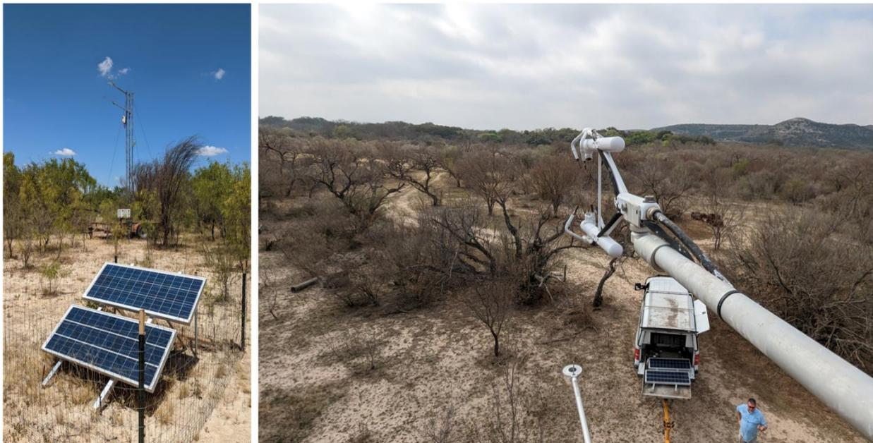
**Figure 2.4. Field Photographs of Uvalde (US-EA5) Station.** (left) Eddy covariance station at the Uvalde site; (right) photograph of the Uvalde site looking approximately into the direction of the sonic azimuth showing general characteristics of mesquite woody savanna ecosystem within measurement footprint (photograph taken in February 2023 during leaf-off conditions).
