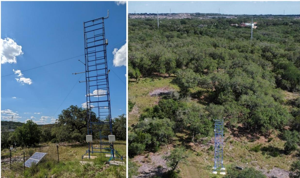
**Figure 2.2 Field Photographs of Cibolo (US-EA4) Site.** (left) Eddy covariance station at the Cibolo site; (right) drone photograph of Cibolo site looking into direction of sonic azimuth showing general characteristics of oak-ashe juniper ecosystem within measurement footprint.
