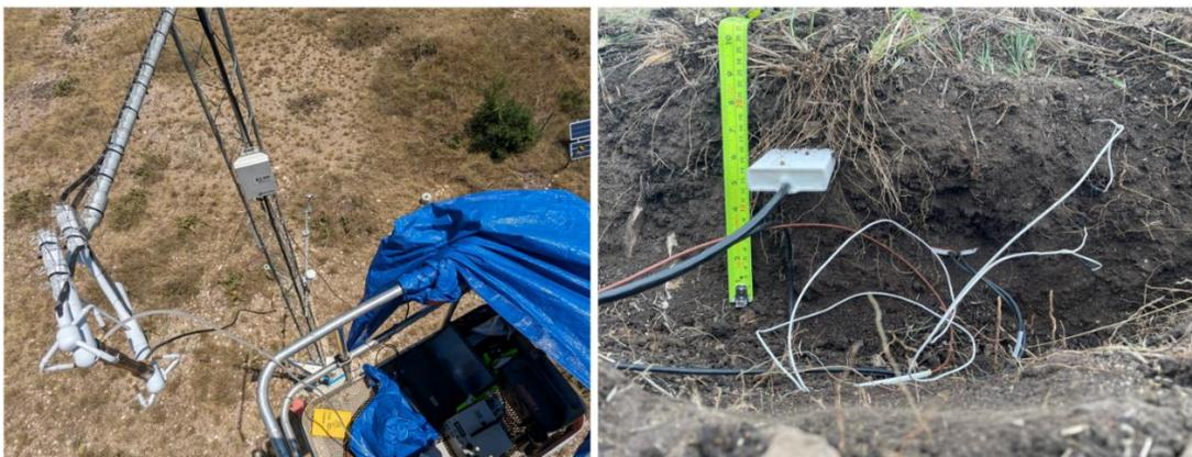
**Figure 2.7. Field Photographs of Nueces (US-EA6) Station Maintenance.** (left) UT-BEG personnel performing a zero-span on the Nueces station IRGASON from a lift; (right) installation of ground-based sensors in soil pit #1 at the Nueces site (right).
